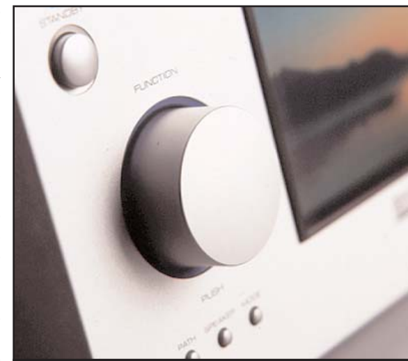
The RSP-1098's front panel carries two large rotary controls: the first adjusts volume, which can be set to change in 1dB, 2dB or 3dB increments; the second to navigate the processor's comprehensive on-screen menus
