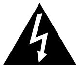
This symbol is to alert the user to the presence of uninsulated dangerous voltages inside the product's enclosure that may constitute a risk of electric shock.
