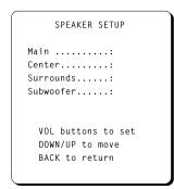
This menu, which is reached from the MAIN menu, allows you to configure the RSP-985 to make optimum use of the capabilities of the speakers in your system. Using these settings, the RSP-985 adjusts its crossovers and digital processing to direct signals to the appropriate speakers.
