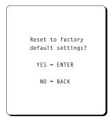
The final menu that can be reached from the SYSTEM SETUP screen is the FACTORY DE-FAULT menu, which resets all system configuration settings to the factory supplied settings.
