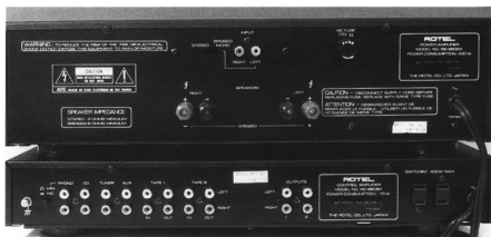
The power amp (above) has a bridged mono input for use with a second power amp, each driving 360 watts into an 8-ohm load at 0.05% THD
